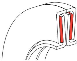
We are using labyrinth seal, which is a mechanical seal that fits around the axle or shaft to prevent the leakage of any particles.
